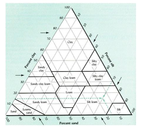
**Figure 8**. The textural class triangle. The arrows outside the arrow show which lines to follow with a given percent of one of the soil separates. In this example follow the dotted lines for a soil with 15% sand, 15% sand and 70% silt and notice that the lines intersect in the silt loam texture class.
