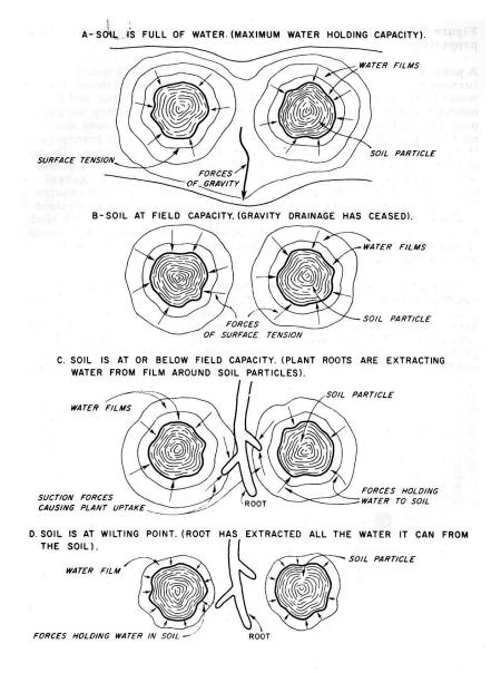
Figure 6.4.--Schematic diagrams of soil-moisture relationships.
