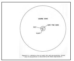
comparison of the size of soil separates is shown in Figure 5.11 (USDA Forest Service, 1961)
