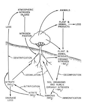
Figure 8.62. -- The nitrogen cycle in soils.
