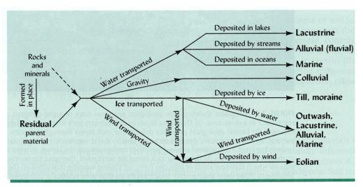
FIGURE 2.10 How various kinds of parent material are formed, transported, and deposited.
