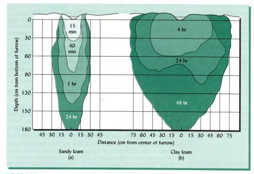
**FIGURE 5.20** Comparative rates of irrigation water movement into a sandy loam and a clay loam. Note the much more rapid rate of movement in the sandy loam, especially in a downward direction. [Redrawn from Cooney and Peterson (1955)]
