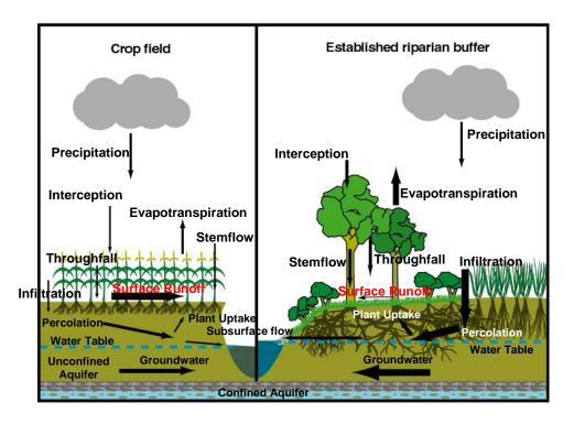
**Figure 11**. Water movement through two similar watersheds under different land-use management. Size of arrows indicate relative differences in volume of water movment.
