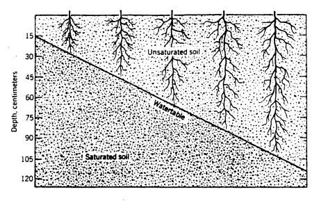
Fig. 5-13 The effect of depth to water table on the length of millet roots. Roots did not enter the saturated soil. (Based on data from Williamson et al., 1969.)
