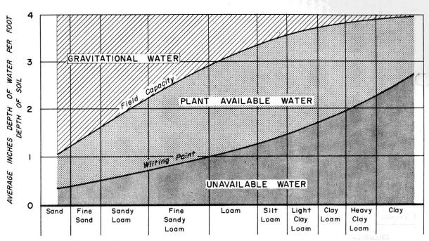
Figure 6.5. -- Typical water characteristics of different-textured soils.
