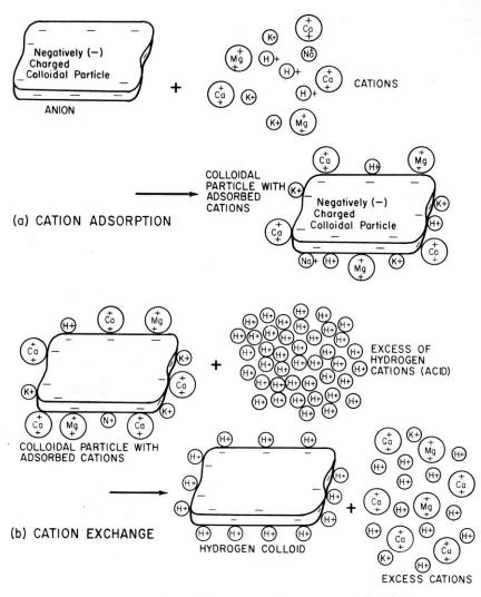
Figure 7.21.--Diagrammatic scheme showing (a) cation adsorption and (b) cation exchange.
