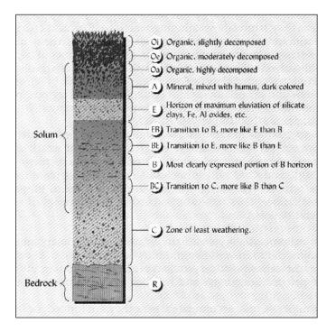
**Figure 1**. Major soil horizons that may be formed in a well-drained soil in the temperate zone. Any particular soil may not have all of these profiles or may have even more detailed sub-horizons and depths of any of the horizons will vary from site to site. The O horizons are not considered part of the mineral soil. The Solum includes the A, E, B and some cemented layers of the C. R layers are consolidated rock, with little evidence of weathering.
