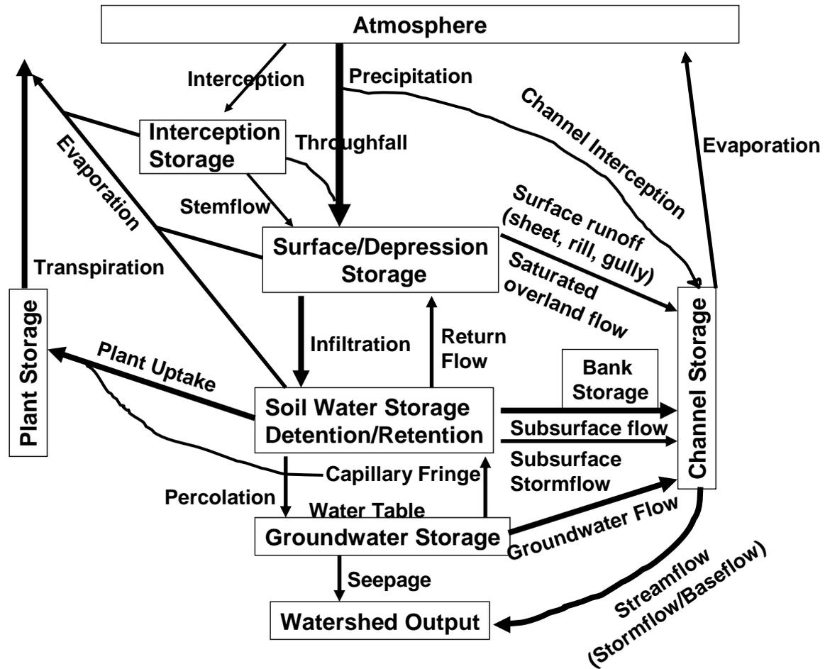
**Figure 10.** The hydrologic cycle showing the role of soil in storage and movement of water through a watershed. The rectangles represent the major water storage sinks in the watershed and the arrows indicate the major pathways of water from one sink to another.
