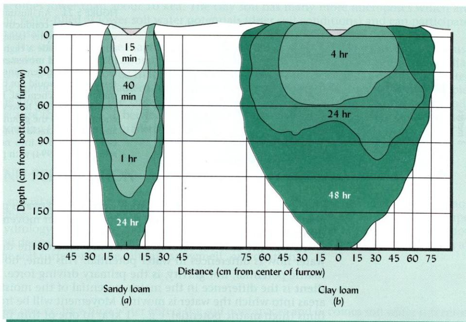
FIGURE 5.20 Comparative rates of irrigation water movement into a sandy loam and a clay loam. Note the much more rapid rate of movement in the sandy loam, especially in a downward direction. [Redrawn from Cooney and Peterson (1955)]
