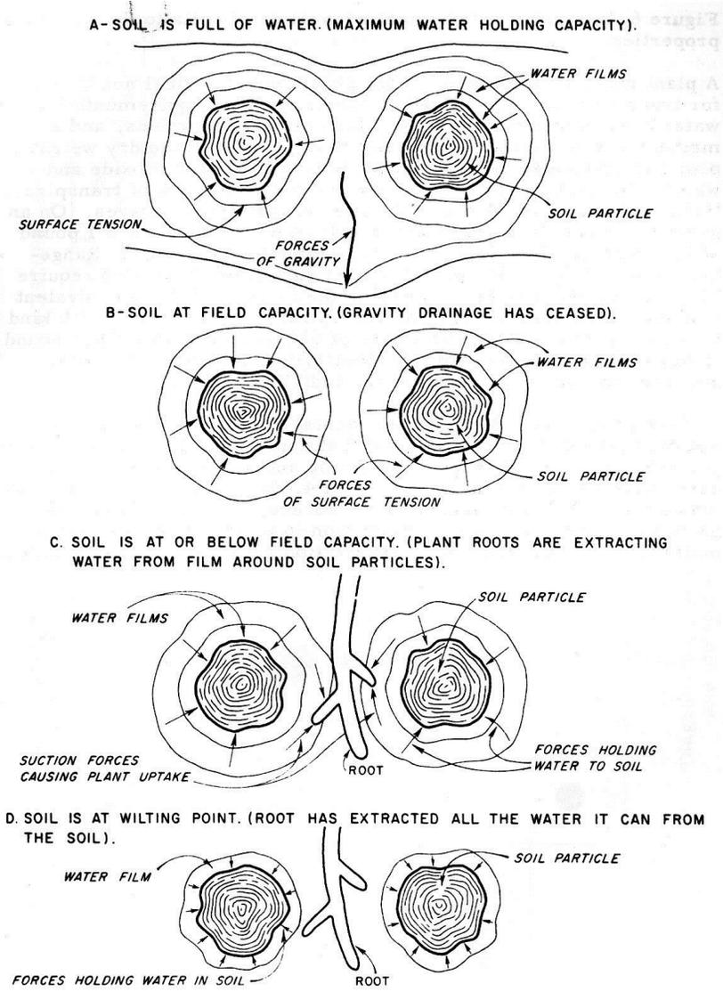
Figure 6.4.--Schematic diagrams of soil-moisture relationships.
