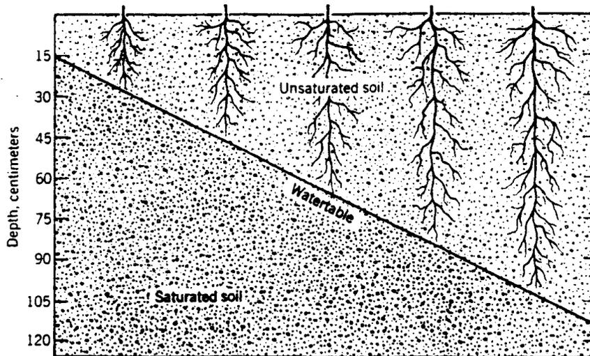
**Fig. 5-13** The effect of depth to water table on the length of millet roots. Roots did not enter the saturated soil. (Based on data from Williamson et al., 1969.)
