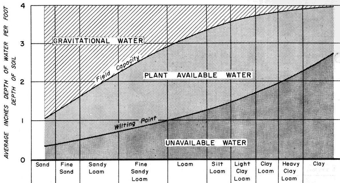
Figure 6.5.--Typical water characteristics of different-textured soils.
